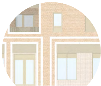
GF Shopfront Brick Surround
