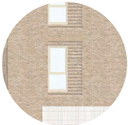
Alternative brick detail - corduroy bricks
