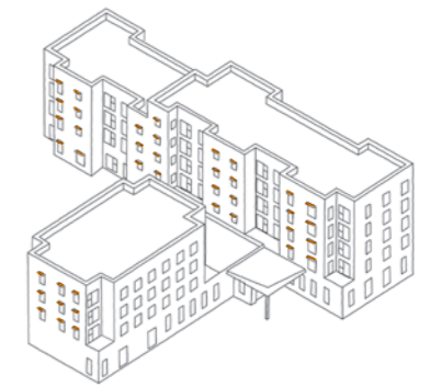
6 Solar shading above balconies and south and west facing windows
